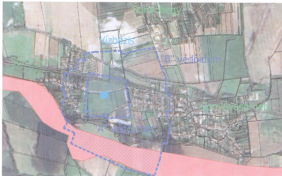
Water abstraction point in Somlóvásárhely showing the penetration of the red mud in the “B” protection zone (Source: Bakonykarszt Viz és Csatornamű plc. water supply and sewage company)
